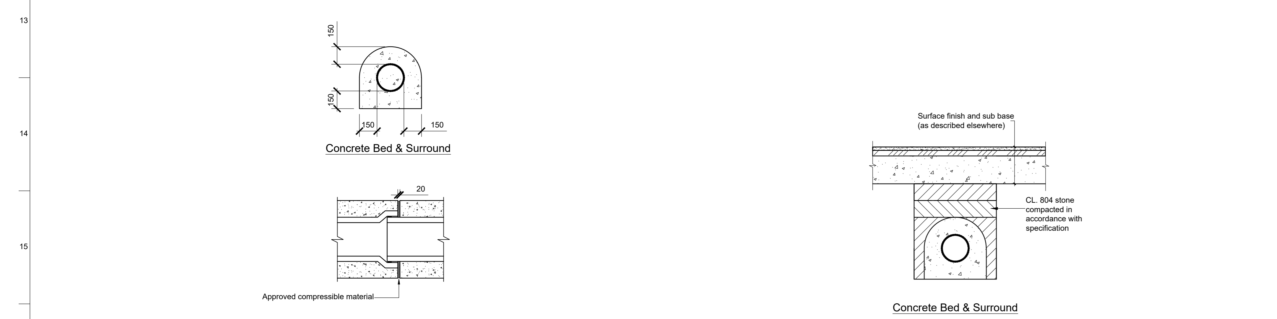
Joint in Concrete Surround to Flexible Jointed Spigot & Socket Pipes Construction Details for Concrete Bed & Surround to Surface Water Drain
